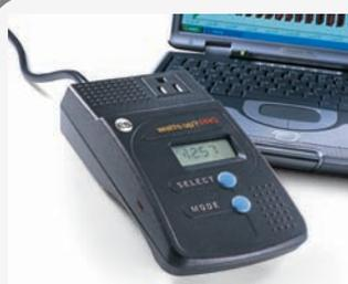
EnergyTeachers.org is now selling data-logging electricity meters at cost. Wondering what's making your electric bill so high? Watts up? Pro is a line of meters from Electronic Educational Devices that can measure many electrical parameters for a device (or a string of devices, up to 15 amps) plugged into it.
