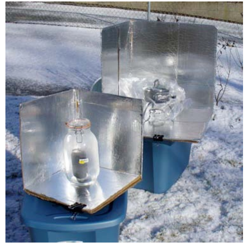
Two solar cookers in below-freezing tests
